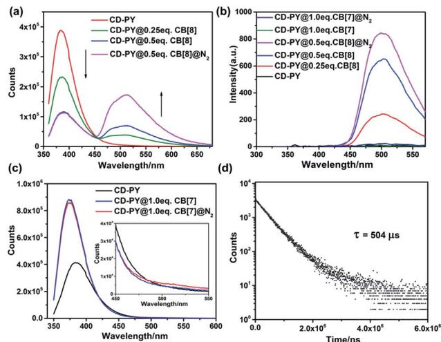
Fig. 2 The prompt photoluminescence (a and c) (inset of (c): the enlarged luminescence peak at 510 nm) and gated (0.1 ms) spectra (b) of CD-PY with or without CB[7,8] and  $N_2$  in aqueous solution. (d) Decay curve of CD-PY@CB[8] (1 : 0.5) aqueous solution at 510 nm ( $[CD-PY] = 0.5 \text{ mM}$ ,  $\lambda_{\text{exc}} = 340 \text{ nm}$ ,  $298 \text{ K}$ ).
