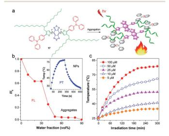
Fig. 7 (a) Schematic illustration for activating intramolecular motion of 17 for boosted photothermal effect. (b) The plot of  $I/I_0$  versus water fraction in H<sub>2</sub>O/THF mixtures. Inset: the photothermal property of 17 NPs. (c) Photothermal conversion behavior of 17 NPs at different concentrations (5–100  $\mu$ M) under 808 nm laser irradiation. Data adapted with permission.<sup>82</sup> Copyright 2019, American Chemical Society.
