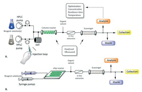
Fig. 1 Schematic representation of a flow reactor configuration involving mesoreactors (A) or microreactors (B). Figure adapted from Tamborini et al.<sup>59</sup>
