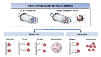
Fig. 3 Scheme of the enzyme immobilization strategies in flow biocatalysis. An example of each type of interaction is also depicted: ionic interaction (adsorption); metal coordination bond (affinity); disulfide bond (covalent reversible); sol-gel matrix (encapsulation); C-N bond (covalent irreversible); CLEAs (crosslinking). Flow reactor: 🐚, enzyme: 🤎, carrier: 🔘.
