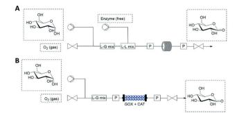
Fig. 6 Flow biocatalysis using pressurized reactors for the O<sub>2</sub> supply. (A) Free enzymes. (B) Packed-bed reactor with co-immobilized enzymes (GOX: glucose oxidase; CAT: catalase).
