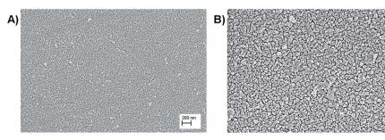
Fig. 2 SEM imagines of PEDOT-C<sub>60</sub> polymer film at different magnifications: (a) 23 000 $\times$ , and (b) 57 000 $\times$ .
