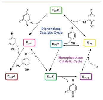
Fig. 2 Catalytic cycle for the hydroxylation of monophenol and the conversion of o-diphenol to o-quinone by the tree types of tyrosinase,  $E_{oxy}$ ,  $E_{met}$ , and  $E_{deoxy}$ .<sup>24</sup>
