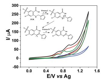
Fig. 6 CVs recorded using different carbon electrodes: (red line) nontreated PDE, (black line) CO2 laser-treated PDE, (blue line) commercial screen-printed carbon electrode, (green line) commercial screenprinted graphene electrode in a solution of 1 mmol  $L^{-1}$  FUR in 0.1 mol L<sup>-1</sup> PBS (pH = 6.8). Inset: schematic representation of FUR oxidation mechanism. Scan rate: 10 mV s<sup>-1</sup>.
