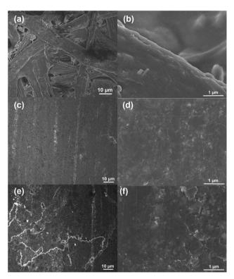
Fig. 2 SEM images with different magnifications of  $1000\times$  and  $20~000\times$ : (a and b) office paper, (c and d) non-treated PDEs, and (e and f) CO<sub>2</sub> laser-treated PDEs.
