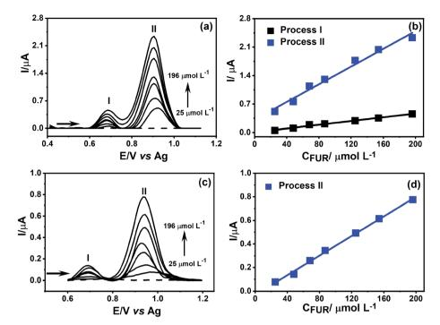
Fig. 7 DPVs recorded using (a)  $CO_2$  laser-treated and (c)  $CO_2$  non-treated PDEs in 0.1 mol  $L^{-1}$  PBS (pH = 6.8) (dashed lines) containing 25, 48, 68, 87, 125, 154, and 196  $\mu$ mol  $L^{-1}$  FUR (solid lines), (b and d) calibration curves obtained from FUR measurements for both  $CO_2$  laser-treated and non-treated PDEs, respectively. Parameters: scan rate: 20 mV s<sup>-1</sup>, amplitude: 50 mV, and step: 10 mV.
