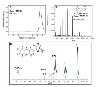
Fig. 2 (A) SEC measurement in THF as an eluent, (B) MALDI-ToF MS, and (C)  $^1$ H NMR analysis of PFB-PEtOx<sub>10</sub>. The SEC trace and the distribution shown in MALDI-ToF indicates a DP10 polymer. In the  $^1$ H NMR, corresponding peaks were labelled, and part of the backbone hydrogens (f) shifted to lower field at around 4.5 ppm from c+d at 3.45 ppm due to initiating group effect.
