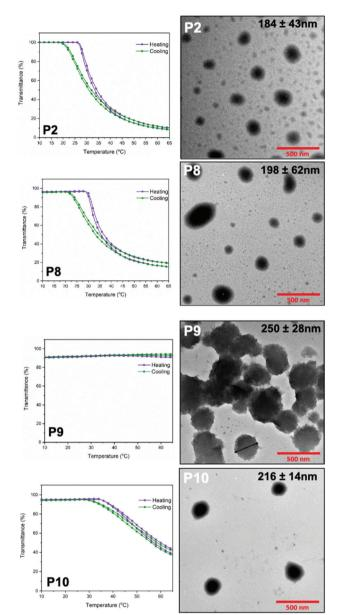
Fig. 5 Transmittance measurements at 550 nM (left) and TEM measurements (right) of P2, P8, P9 and P10.
