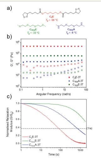
Fig. 4 (a) Structures of monomers to make networks at 8:1 ratio. (b) Rheology frequency sweep of networks at 25 °C (1% strain from 0.1 to 10 Hz, or 0.06 to 62 rad s<sup>-1</sup>). (c) Stress relaxation experiments at 2% strain, 100 °C.
