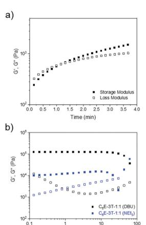
Fig. 2 (a) Rheology time sweep (10% strain, frequency of 1 Hz) at 25 °C to characterise gelation time of C<sub>6</sub>E-3T-1:1 using 1 mol% DBU. (b) Frequency sweep analysis showing storage and loss modulus versus frequency for networks synthesized using DBU or NEt<sub>3</sub> at 25 °C (1% strain from 0.1 to 10 Hz, or 0.06 to 62 rad  $s^{-1}$ ).
