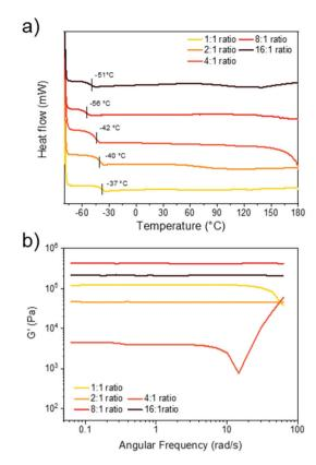
Fig. 3 Thermal and rheological properties of C<sub>6</sub>E-3T networks. (a) DSC thermograms of the 2nd heating cycle from -80 to 180 °C, 10 °C min<sup>-1</sup> (b) Frequency sweep analysis of films showing storage modulus versus frequency at 25 °C (1% strain from 0.1 to 10 Hz, or 0.06 to 62 rad  $s^{-1}$ ).
