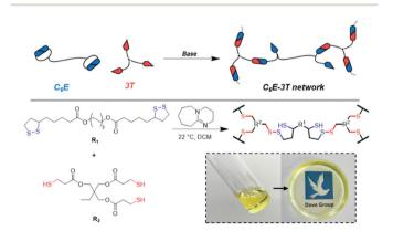
Fig. 1 Schematic illustrating the synthesis of disulfide-based CAN (C<sub>6</sub>E-3T) assuming 1:1 disulfide to thiol. Inset shows photograph of monomer solution and subsequent crosslinking to afford homogeneous film after solvent evaporation.
