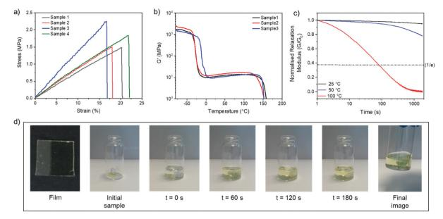
Fig. 5 Thermomechanical and physical data for C6E-3T-8:1. (a) Uniaxial tensile testing at 22 °C, 10 mm min<sup>-1</sup> strain rate. (b) DMA temperature sweep from -80 to 180 °C, 5 °C min<sup>-1</sup>. (C) Stress relaxation experiments at 2% strain (25 °C, 50 °C, and 100 °C). (d) Chemical recycling of as-synthesised film cut into small pieces (200 mg film in 5 mL DCM solution, 0.01 M DBU).
