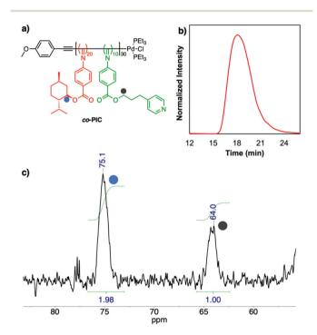
Fig. 1 (a) Structure of the side-chain functionalized helical co-PIC with dots highlighting backbone signals of interest in the <sup>13</sup>C NMR spectrum. (b) SEC curve of co-PIC showing number average molecular weight  $(M_n)$ of 7200 and dispersity (D) of 1.44. (c) Partial <sup>13</sup>C NMR spectrum (600 MHz, CD<sub>2</sub>Cl<sub>2</sub>) of co-PIC showing backbone signals from two types of monomers. Integration of these signals confirms that the ratio of chiral to achiral component is 2:1.
