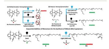
The switchable copolymerization converting from coordinationinsertion polymerization of hexene to radical polymerization of methacrylate in one shot under visible light irradiation. Reproduced from ref. 31 with permission from the American Chemical Society, copyright 2018.
