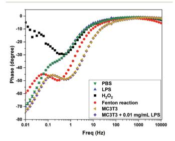
Fig. 7 Phase shifts in Bode plots for the electrochemical impedance spectroscopy (EIS) results obtained with the 0.64 wt% Ce/Carbonmodified electrode in the presence of PBS, LPS, H<sub>2</sub>O<sub>2</sub>, Fenton reaction, MC3T3, and MC3T3 + LPS (additional induced oxidative stress).
