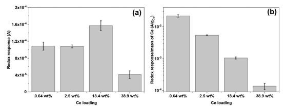
Fig. 6 (a) Redox response obtained with the different CeO<sub>x</sub> nanoclusters/carbon composites toward 10 mM of 'OH (Fenton reaction) and (b) redox response normalized per mass of cerium on the composite. The error bars represent the standard deviation of three repetitive measurements.
