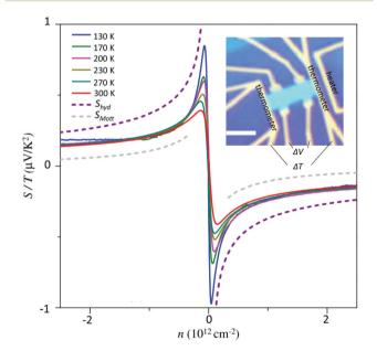
Fig. 15 Measured  $S/T_e$  as a function of charge carrier density n at different temperatures. The grey and purple curves represent  $S_{Mott}/T_{e}$ and  $S_{hyd}/T_e$ , respectively. The inset shows a typical device used to measure S, where the scale bar corresponds to 2  $\mu m$ . The figure is adapted with permission from ref. 190 (Copyright 2016 American Physical Society).
