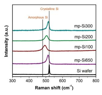
Fig. 3 Raman spectra of Si wafer and mp-Si NPs prepared under different magnesiothermic reduction conditions. mp-Si650 was prepared using the single step heating at 650 °C for 3 h. mp-Si100, mp-Si200, and mp-Si300 were prepared using the two step heating method with the second annealing temperature of 100, 200, and 300 °C, respectively.
