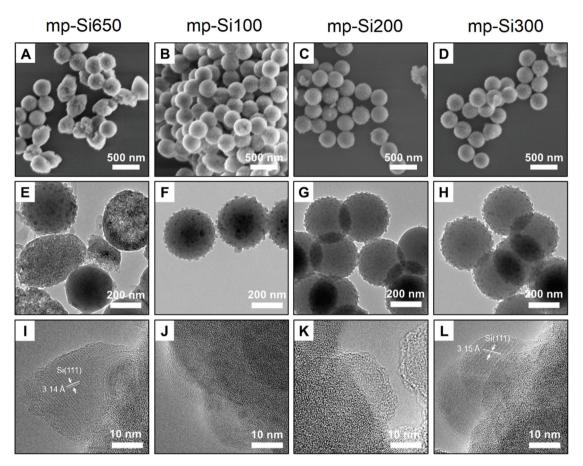
Fig. 2 (A–D) SEM, (E–H) TEM, and (I–L) HRTEM images of mp-Si NPs prepared under different magnesiothermic reduction conditions. mp-Si650 was prepared using the single step heating at 650 °C for 3 h. mp-Si100, mp-Si200, and mp-Si300 were prepared using the two step heating method with the second annealing temperature of 100, 200, and 300 °C, respectively.
