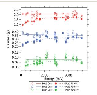
Fig. 6 The corrected (open symbols) and uncorrected (closed symbols) masses of the element Ca in the active measurement volume. The corrected mass values from analytical peaks at various gamma energies show no energy-dependent tendency and agree within the 1-sigma statistical uncertainty, calculated as described in ref. 24. The interpolation curves were determined with a nonlinear weighted least-squares fit.
