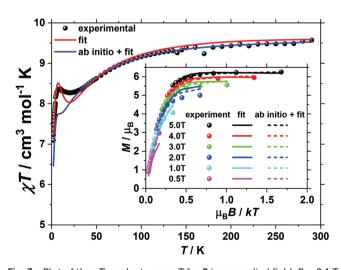
Fig. 3 Plot of the  $\chi T$  product *versus T* for 2 in an applied field,  $B=0.1\,\mathrm{T}$ . Inset: Plot of the magnetisation *versus* field data for 2. The solid and dashed lines are fits of the experimental and *ab initio* data, as described in the text.
