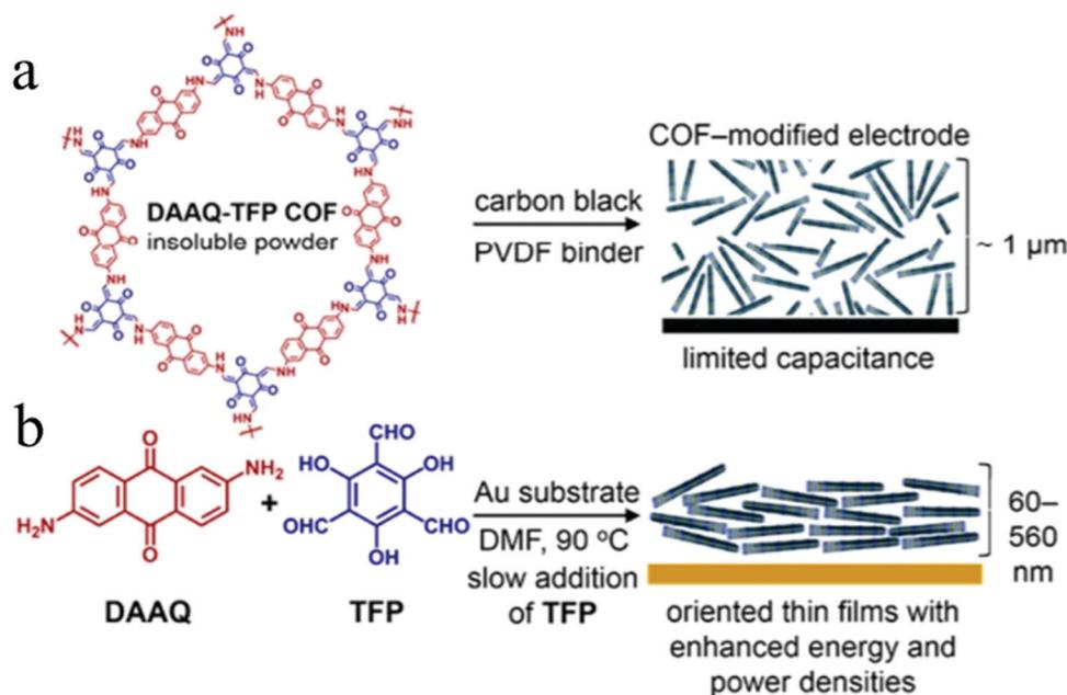
Fig. 14 (a) Structure of DAAQ–TFP COF with random orientation on the electrode; (b) schematic illustration of the DAAQ–TFP COF as an oriented thin film on an electrode surface. Reproduced from ref. 219 with permission from the American Chemical Society, copyright 2015.
