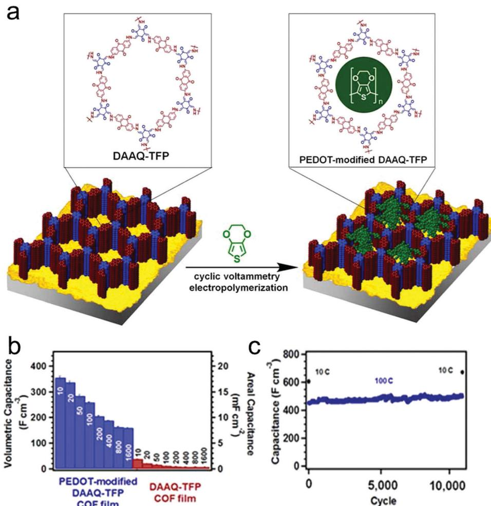
**Fig. 15** (a) Schematic representation of the synthesis of PEDOT-modified DAAQ-TFP COF film; (b) average capacitance of PEDOT-modified DAAQ-TFP and DAAQ-TFP at different charging rates; (c) extended cycling of PEDOT-modified DAAQ-TFP film showing stability over 10 000 cycles. Reproduced from ref. 96 with permission from the American Chemical Society, copyright 2016.
