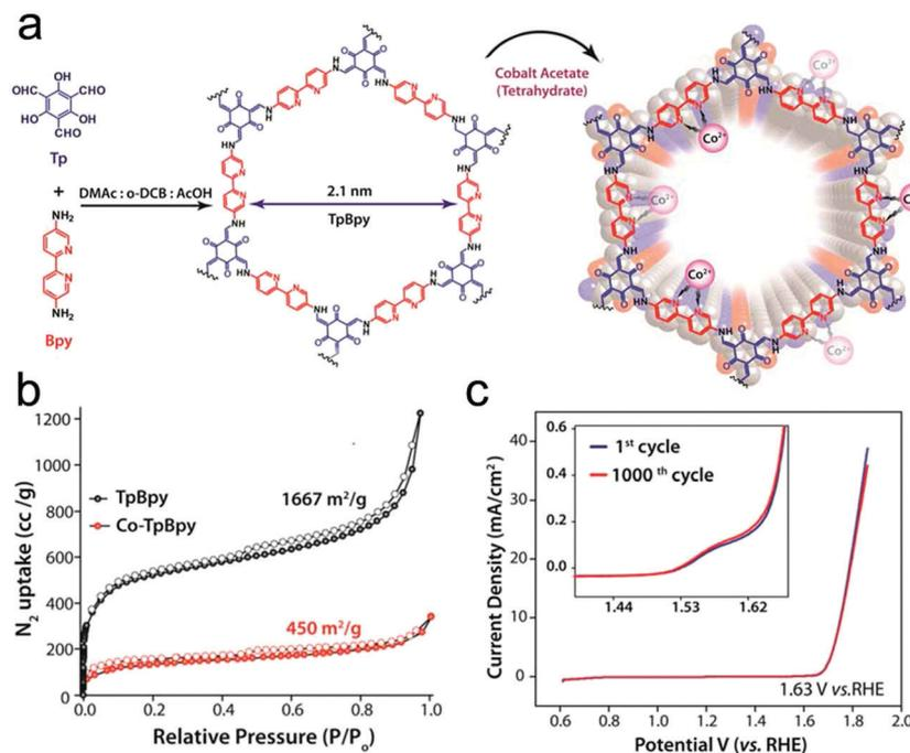
Fig. 7 (a) Schematic illustration of TpBpy and Co-TpBpy with Co incorporation; (b)  $\text{N}_2$  sorption isotherms of TpBpy (black) and Co-TpBpy (red); (c) LSV profiles of Co-TpBpy before and after 1000 cycles from 0.6 V to 1.8 V in a phosphate buffer (pH 7.0). Inset: An enlarged view of the LSV profile. Reproduced from ref. 55 with permission from the American Chemical Society, copyright 2016.
