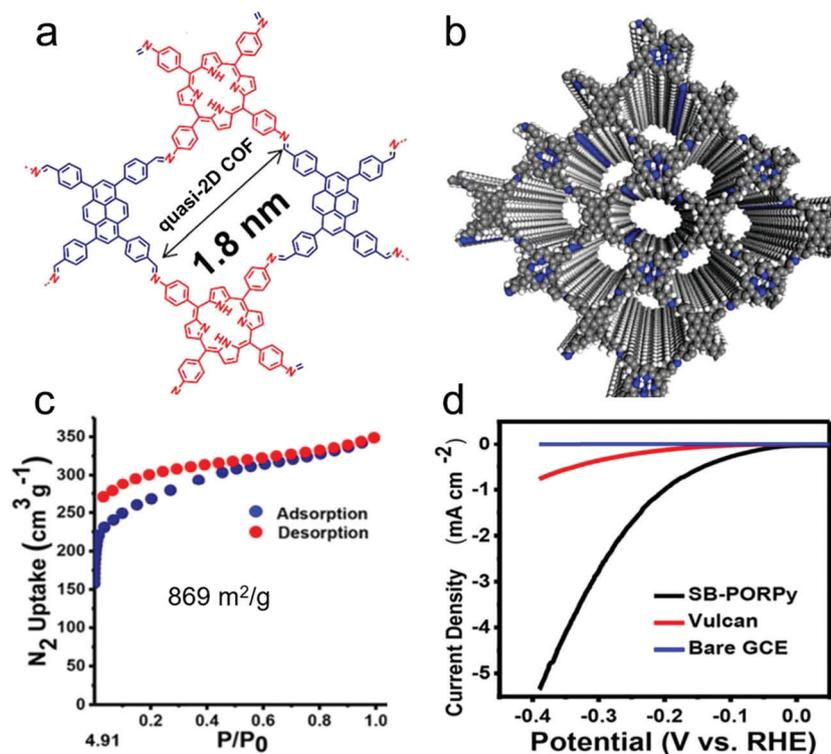
Fig. 5 (a) Topological structure of SB-PORPy COF; (b) simulated structure of SB-PORPy COF; (c)  $\text{N}_2$  sorption isotherm at  $77 \text{ K}$  of SB-PORPy COF; (d) linear sweep voltammetry (LSV) profile of the SB-PORPy COF electrode compared to those of the bare glassy carbon electrode (GCE) and Vulcan. Reproduced from ref. 101 with permission from the American Chemical Society, copyright 2017.
