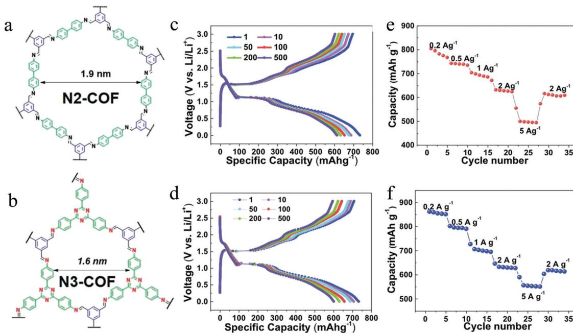
Fig. 18 Structures of (a) N2-COF and (b) N3-COF; charge–discharge cycles at  $1 \text{ A g}^{-1}$  of (c) N2-COF and (d) N3-COF; chemical stability tests at different current densities ( $0.2\text{--}5 \text{ A g}^{-1}$ ) of (e) N2-COF and (f) N3-COF. Reproduced from ref. 245 with permission from the Royal Society of Chemistry, copyright 2016.
