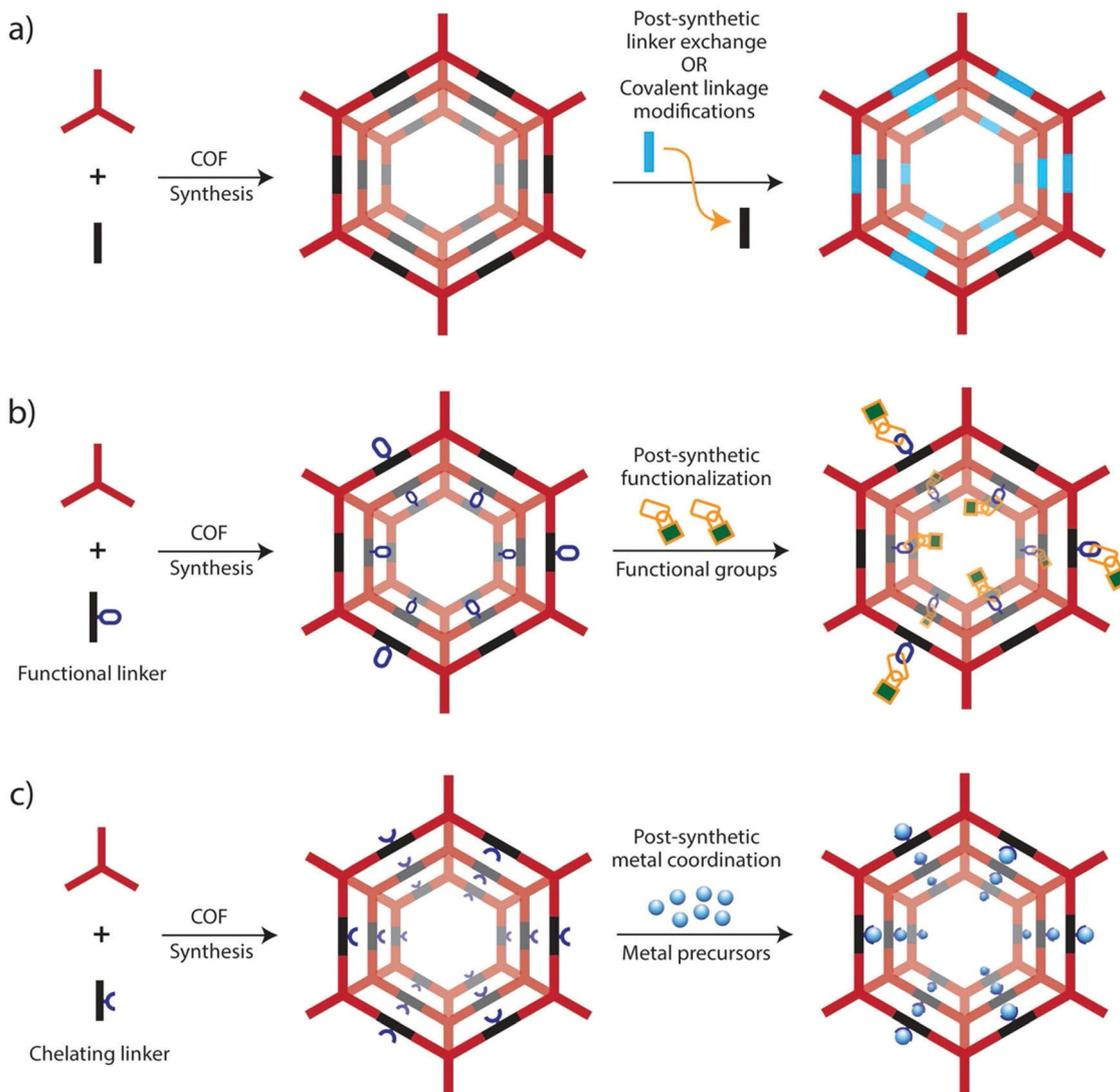
Fig. 3 Strategies for the preparation of functional COFs via post-synthetic modification (PSM) for their applications in electrocatalysis and energy conversion and storage.
