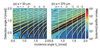
Fig. 3 Contour plots composed of diffraction patterns measured at various incidence angles with two complementary gratings of (a)  $a=30~\mu m$  and (b) 370  $\mu m$ . The vertical dashed white lines indicate the Rayleigh incidence angle  $\theta_{R,m}$  where the mth-order diffraction beam emerges from the grating. The continuous grey lines present the calculated diffraction angles
