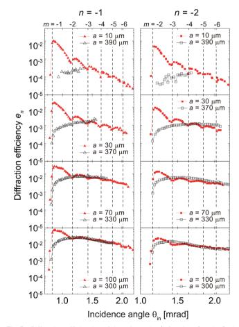
Fig. 5 Diffraction efficiencies of the -1st-order (left column) and -2ndorder (right column) plotted as a function of incidence angle  $\theta_{in}$ . The dashed vertical lines indicate Rayleigh angles of emergence of another diffraction beam of order m as labeled on top of the graphs
