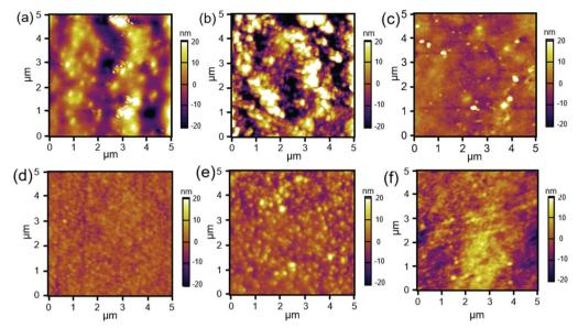
AFM height micrographs of (a) SF<sub>EO</sub>, (b) SF<sub>EO</sub>-zwitter, (c) SF<sub>EO</sub>-PEG, (d) SF<sub>OX</sub>, (e) SF<sub>OX</sub>-zwitter, and (f) SF<sub>OX</sub>-PEG film surfaces.
