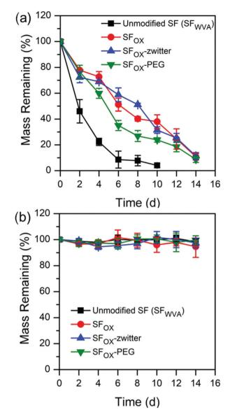
Fig. 4 Degradation profiles of water annealed silk ( $SF_{WVA}$ ), hydroxylated silk ( $SF_{OX}$ ), and the silk brush-like polymer films in (a) 1 U mL<sup>-1</sup> protease XIV and (b) 1X PBS, at 37 °C.
