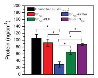
Fig. 5 Amount (ng cm<sup>-2</sup>) of bovine serum albumin (BSA) adsorbed onto unmodified silk, oxidized silk, and silk brush-like polymer surfaces normalized to film area. \* denotes significance at p < 0.05.
