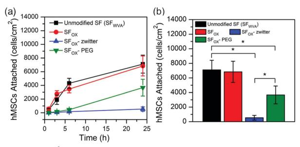
Fig. 6 Attachment (cells per cm<sup>2</sup>) of human mesenchymal stem cells (hMSCs) to unmodified silk, oxidized silk, and silk brush-like polymer surfaces normalized to film area at (a) 1 h, 3 h, 6 h, and 24 h; and (b) 24 h. \* denotes significance at p < 0.05.
