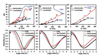
Fig. 5 (a–c) QCM-D  $\Delta D/\Delta f$  plots (7th overtone) and (d and e) SPR reflectivity curves (d–f) showing the interaction of CD44-his tag protein with electrostatically deposited and crosslinked (PLL-HA) $_5$  films assembled from HA of different size, *i.e.* (a and d) 6.4, (b and e) 752 and (c and f) 1500 kDa. In the SPR curves, the black dashed line represents the normalized angle shift of (PLL-HA) $_5$ , *i.e.* the SPR signal of the construct alone.
