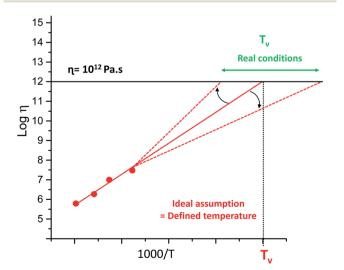
Fig. 9 Example of imperfect evaluation of the topology freezing temperature  $(T_{\nu})$  caused by measurement errors, based on standard deviations and small temperature window or unconsidered low temperature interactions.
