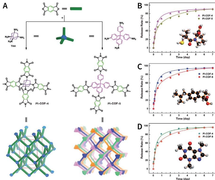
Fig. 65 3D polyimide COFs for drug loading and release. (A) Preparing 3D PI-COF-4 and PI-COF-5. (B) Release profile of captopril-loaded 3D COFs. (C) Release profile of ibuprofen-loaded 3D COFs. (D) Release profile of caffeine-loaded 3D COFs. Adapted with permission.<sup>97</sup> Copyright 2015, American Chemical Society.
