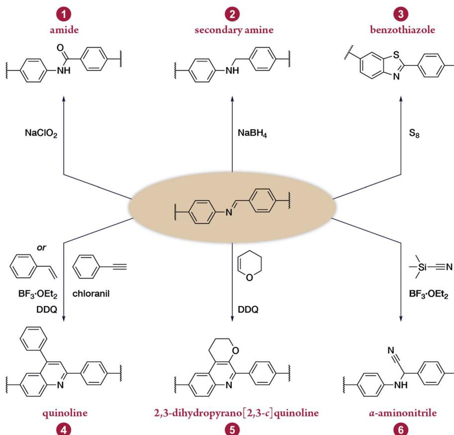
Fig. 55 Post-synthesis linkage conversion of C=N-linked COFs.
