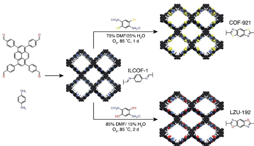
Fig. 61 Combining monomer exchange with linkage transformation to synthesize thiazole-linked COF-921 and oxazole-linked LZU-192 COFs. Adapted with permission.<sup>345</sup> Copyright 2018, American Chemical Society.
