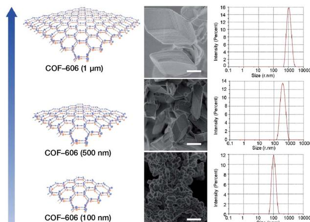
Fig. 29 COF-606 with different particle sizes measured by SEM and DLS. Scale bar: 500 nm. Adapted with permission.<sup>198</sup> Copyright 2020, Elsevier Inc.
