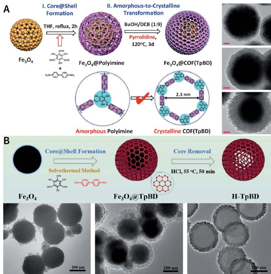
Fig. 38 (A) Preparation protocol and HRTEM images of  $\text{Fe}_3\text{O}_4$ @COF (TpBD) with shell thicknesses of 20, 50, and 100 nm. Scale bar: 50 nm. Adapted with permission.<sup>232</sup> Copyright 2016, Wiley-VCH Verlag GmbH & Co. KGaA, Weinheim. (B) Synthesis protocol and HRTEM images of hollow COF nanoshells. Adapted with permission.<sup>233</sup> Copyright 2018, Elsevier B.V.
