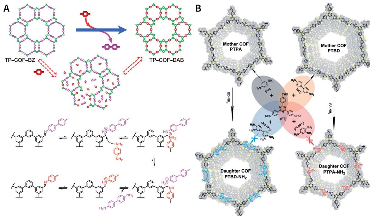
Fig. 60 (A) COF-to-COF transformation via heterogeneous monomer exchange. Adapted with permission.<sup>343</sup> Copyright 2017, American Chemical Society. (B) COF-to-COF transformation for the preparation of *de novo* unreachable amino-functionalized PTBD-NH<sub>2</sub> and PTPA-NH<sub>2</sub> COFs. Adapted with permission.<sup>344</sup> Copyright 2018, The Royal Society of Chemistry.
