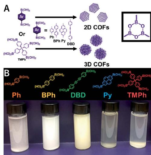
Fig. 35 Synthesis of boroxine-linked 2D and 3D COFs in acetonitrile/1,4-dioxane/mesitylene (5 : 4 : 1, v/v/v). Adapted with permission.<sup>218</sup> Copyright 2019, American Chemical Society.
