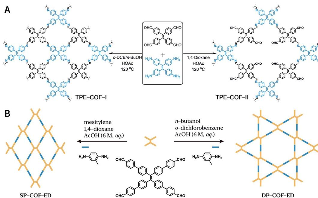
Fig. 9 Solvent-induced constitutional isomerism of COFs. (A) Preparation of TPE-COF-I with conventional [4 + 4] pathway and TPE-COF-II with unusual [4 + 2] pathway. Adapted with permission.<sup>100</sup> Copyright 2018, American Chemical Society. (B) Synthesis of SP-COF-ED with square monoporous structure and DP-COF-ED with triangular and hexagonal dual-porous structures.
