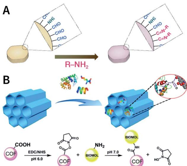
Fig. 52 (A) BDF of imine-linked COFs. (B) Grafting biomolecules on the surface of NKCOF-1 COF containing carboxyl groups *via* BDF. Adapted with permission.<sup>323</sup> Copyright 2018, Wiley-VCH Verlag GmbH & Co. KGaA, Weinheim.
