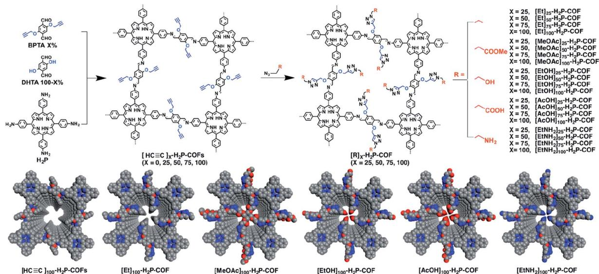
Fig. 44 Post-SM of porphyrin-based COFs with various functional groups *via* click reactions. Adapted with permission.<sup>289</sup> Copyright 2015, American Chemical Society.
