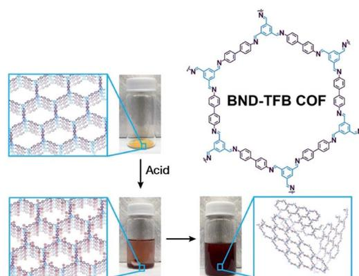
Fig. 27 Charge-mediated self-exfoliation of BND-TFB COF via trifluoroacetic acid treatment. Adapted with permission.<sup>194</sup> Copyright 2020, Wiley-VCH Verlag GmbH & Co. KGaA, Weinheim.
