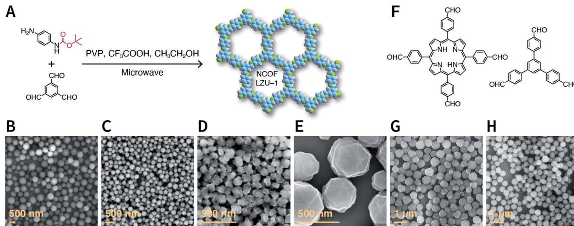
Fig. 33 Synthesis of NCOFs using *tert*-butyl (4-aminophenyl)carbamate as the precursor. (A) Synthesis of NCOF LZU-1. (B–D) LZU-1 nanocrystals with different particle sizes. (E) Hexagonal LZU-1 nanocrystals. (F) Aldehydes for the synthesis of nanoscale Por-COF and TFPB-PDA-COF. (G) Por-COF nanocrystals. (H) TFPB-PDA-COF nanocrystals. Adapted with permission.<sup>215</sup> Copyright 2017, American Chemical Society.
