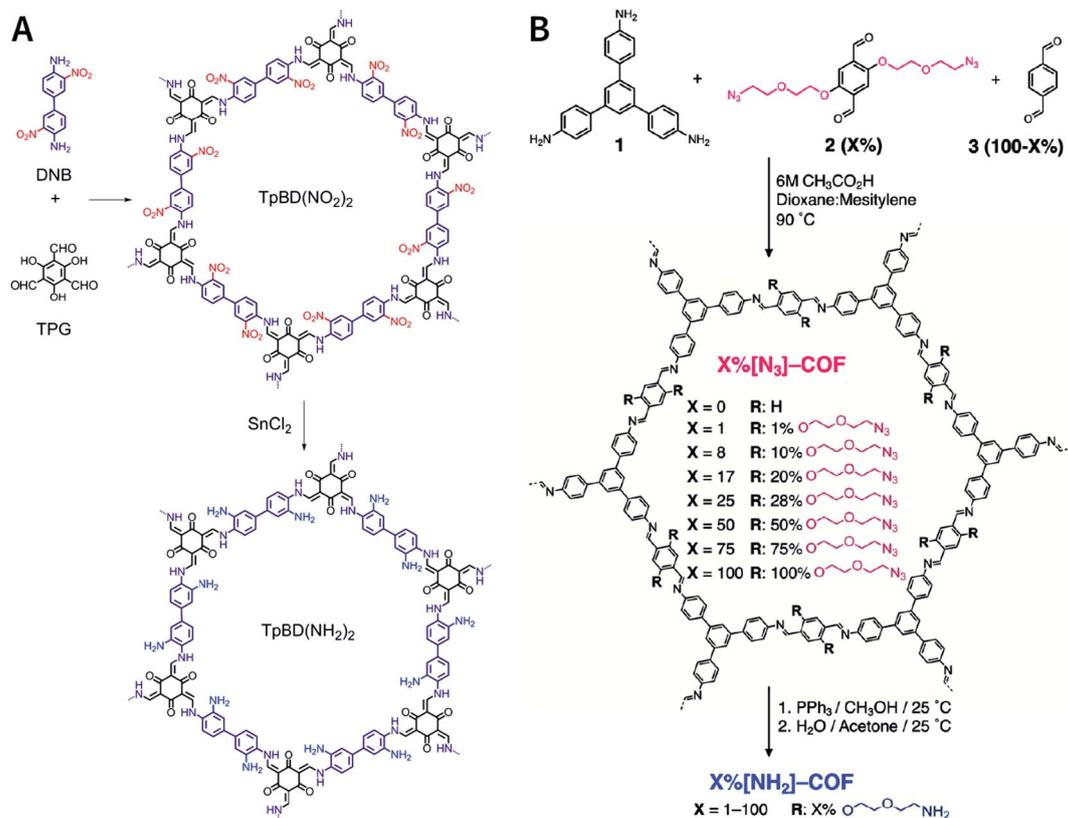
Fig. 50 Inserting amino groups into COFs by the reduction of nitro and azide groups. (A) Adapted with permission.<sup>312</sup> Copyright 2016, American Chemical Society. (B) Adapted with permission.<sup>314</sup> Copyright 2018, American Chemical Society.
