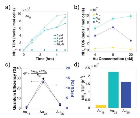
Fig. 4 Light-driven biocatalytic reaction efficiency using nanorgs from different Au NCs. (a) Time-dependent ammonia production with Au<sub>22</sub> NC-nanorgs. (b) A 3D plot showing the ammonia turnover number using nanorgs made from different Au NCs at different concentrations. (c) Calculated quantum efficiency (QE) and photon-to-fuel conversion efficiency (PFCE) of each optimized nanorgs. (d) Ammonia turnover frequency using nanorgs made from different Au NCs (8 µM).
