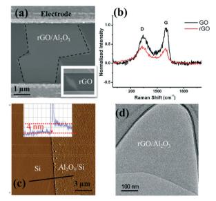
Fig. 3 (a) SEM image of the  $Al_2O_3$  film covering the rGO sheet. Inset: rGO sheet spans across the interdigitated electrode gap and is transparent under the electron beam. (b) Raman spectra of GO (black) and rGO (red). (c) AFM image of the  $Al_2O_3$  film; the solid black line indicates the scanning trace; inset: height profile. (d) TEM image of the  $Al_2O_3$  film covering the rGO nanosheet.
