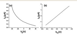
Fig. 2 (a) Field-effect characteristics of rGO was tested with a backgate voltage from -40 to 40 V, with a 0.1 V bias voltage loaded between the source and the drain electrodes. The identified current on/off ratio is  $\sim 1.4$ . (b) I-V characterization of rGO with the source drain voltage from -0.5 to 0.5 V.
