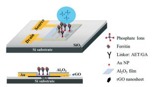
Fig. 1 Schematic diagram and side view of the rGO-based FET device for phosphate ion detection. The gaps between the interdigitated Au electrodes are bridged by single-layer rGO nanosheets. The sensing area is covered by a thin  $Al_2O_3$  film ( $\sim 4$  nm) with surface-deposited Au NPs ( $\sim 4$  nm diameter). The ferritin probes were immobilized on Au NPs with an AET/GA linker.
