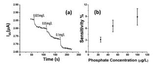
Fig. 6 (a) Dynamic responses of the rGO-FET sensor to phosphate ions with concentrations of 25  $\mu g$  L<sup>-1</sup>, 50  $\mu g$  L<sup>-1</sup>, and 100  $\mu g$  L<sup>-1</sup>. (b) The relationship between the phosphate concentration and the corresponding sensitivity shown by the sensing platform. The lower detection limit could reach down to 10  $\mu$ g L<sup>-1</sup>.
