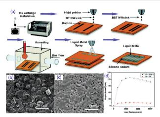
Fig. 8 (a) Fabrication schematic for the development of the inkjet-printed TEG device; SEM micrographs of the printed BST50 (b) and BT50 (c) nanowires annealed at 450 °C for 10 min; (d) output power of the printed TEG as a function of load resistance. (Reproduced from ref. 103 with permission from The Royal Society of Chemistry.).
