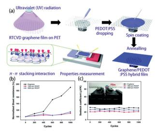
Fig. 12 (a) Schematics of the hybridization process of RTCVD graphene and PEDOT:PSS and the  $\pi$ - $\pi$  stacking interaction interface between graphene and the PEDOT:PSS chains. (b) Plots of the sheet resistance and (c) Seebeck coefficient versus the bending cycle number of the graphene film and RCG/P hybrid films. (Reproduced from ref. 149 with permission from AIP.).
