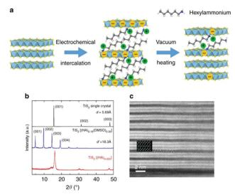
Fig. 2 (a) Schematic of the electrochemical intercalation process. (b) XRD patterns of TiS2 single crystal and its related superlattice structures. (c) Magnified STEM image of TiS<sub>2</sub>(HA)<sub>0.025</sub>. (Reproduced from ref. 33 with permission from Nature Communication )
