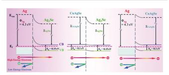
Fig. 3 Equilibrium band diagrams for Ag/Ag<sub>2</sub>Se, CuAgSe/Ag<sub>2</sub>Se and Ag/ CuAqSe.38
