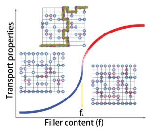
Fig. 1 Percolation theory and nonlinear changes in the transport properties of composites near the percolation threshold  $f_{\rm c}$  (dashed blue line). The insets show the geometric phase transition of fillers (denoted by dark spots) in the microstructures of the composites near percolation.
