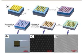
Fig. 9 (a) Scheme of the fabrication of the organic/inorganic hybrid film via by nanosphere lithography, (b) digital photograph of closely packed monolayer PS nanospheres on a SiO<sub>2</sub>/Si substrate after etching, SEM image of (c) Bi<sub>2</sub>Te<sub>3</sub> nanoparticle arrays prepared by using 100 nm PS nanospheres as patterns and (d) PEDOT/Bi<sub>2</sub>Te<sub>3</sub>(100) hybrid films. <sup>109</sup>
