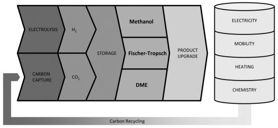
Fig. 2 Power-to-X pathways to transform electricity to chemicals *via* electrolysis and synthesis. The power-to-X principle connects different energy sectors *via* carbon capture from industrial plants or chemical/natural (photosynthesis) CO<sub>2</sub> scrubbing from the air, the carbon cycle can be closed so that no additional CO<sub>2</sub> is emitted. This paper regards paths to transform electricity to liquid fuels for the mobility sector.
