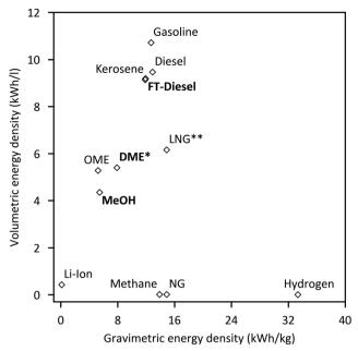
Fig. 1 Gravimetric and volumetric energy density of different fuels and Li-Ion batteries for comparison (\*at 10 bar; \*\*at -160 °C).  $^{13-15}$
