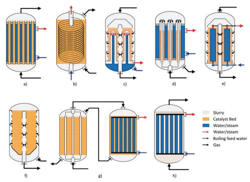
Fig. 6 Simplified reactor layout of (a) Lurgi tubular reactor, (b) Linde Variobar, (c) Toyo MRF, (d) Mitsubishi Superconverter, (e) Methanol Casale IMC, (f) Haldor Topsøe adiabatic reactor, (g) Lurgi MegaMethanol and (h) Air Products LPMEOH, adapted from Buttler 2018.<sup>138</sup>
