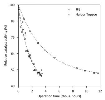
Fig. 14 Deactivation of direct DME synthesis catalysts of Haldor Topsøe $^{130}$  and JFE (260  $^{\circ}$ C, 50 bar). $^{258}$
