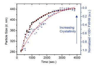
**Fig. 2** Relationship between particle size and crystallinity in terms of FWHM with respect to time. Curve fit (red) illustrates the different rate constants of the polymerization and crystallization processes.
