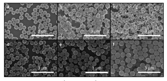
Fig. 4 SEM images of colloidal suspension at 50 equiv.  $h^{-1}$  (a-c) and 1 equiv.  $h^{-1}$  (d-f) of monomer addition. Aliquots were drop-casted after (a, d) 2 equivalents, (b, e) 4 equivalents, and (c, f) 6 equivalents of monomers were added.
