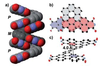
Fig. 3 Structure of PPDH from SCXRD. Free solvent, the  $CH(C_5H_{11})_2$  chains, and hydrogen atoms have been hidden to provide an unobstructed view of the aryl surface. Thermal ellipsoids are set at 30% probability. (a) The racemate assembles as heterochiral columns in the solid state. Extensive intramolecular overlap between the PDI subunits (b) distorts their perylene cores into shallow bowls (c).
