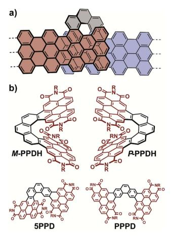
Fig. 1 (a) The fusion of two armchair nanographenes with phenanthrene provides a  $\pi$ -extended bilayer helicene. (b) Fusion with two PDI subunits via oxidative photocyclization at elevated temperatures overwhelmingly favors the formation of PPDH over its isomers, 5PPD and PPPD.
