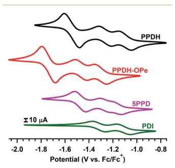
Fig. 4 Cyclic voltammograms of PPDH, PPDH-OPe, 5PPD, and monomeric PDI (1 mM, 50 mV s<sup>-1</sup> scan rate) in Ar-sparged DCM with  $0.1\ M\ [Bu_4N][PF_6]$  as the supporting electrolyte. For all species, R = $CH(C_5H_{11})_2$
