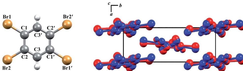
Fig. 1 Molecular structure of a TBB molecule (left) and the packing differences between the two TBB polymorphs,  $\beta$ -TBB (blue) and  $\gamma$ -TBB (red).
