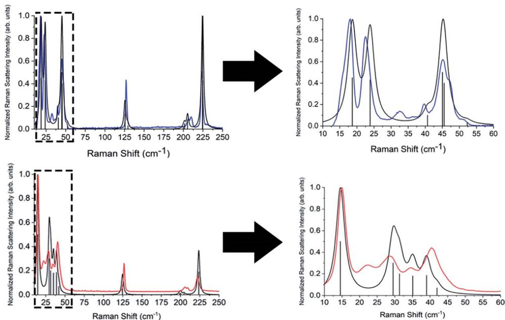
Fig. 6 Experimental Raman spectra for  $\beta$ -TBB (blue) at 107 K and  $\gamma$  (red) at 318 K with their corresponding simulated (black) Raman spectra. The boxed areas in the lower frequency range (left) are shown expanded on the right.
