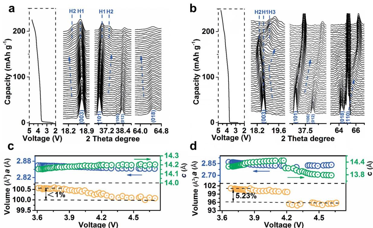
Fig. 4 Structural evolution of LiNi<sub>0.9</sub>Co<sub>0.07</sub>Mg<sub>0.03</sub>O<sub>2</sub> (a and c) and NCM811 (b and d). (a and b) *In situ* XRD patterns at selected 2θ regions and the corresponding galvanostatic curves on first charging. (c and d) The variation of lattice parameters and cell volumes as a function of voltage.
