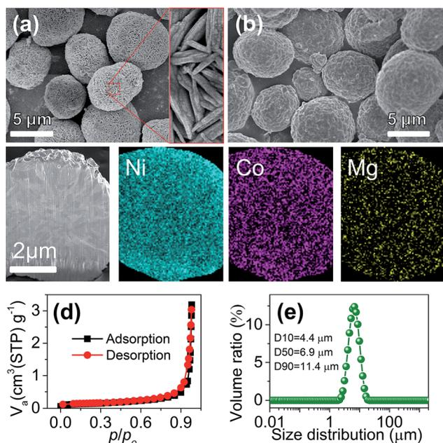
Fig. 1 (a) SEM images of the  $\text{Ni}_{0.9}\text{Co}_{0.07}\text{Mg}_{0.03}(\text{OH})_2$  precursor. (b) SEM image, (c) cross-sectional elemental mapping, (d)  $\text{N}_2$  adsorption/desorption isotherms and (e) particle size distribution of the synthesized  $\text{LiNi}_{0.9}\text{Co}_{0.07}\text{Mg}_{0.03}\text{O}_2$ .
