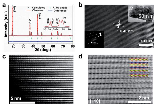
Fig. 2 (a) Rietveld refined XRD pattern of the prepared  $\text{LiNi}_{0.9}\text{Co}_{0.07}\text{Mg}_{0.03}\text{O}_2$ . (b) HRTEM image. Insets in (b) show the SAED pattern (1) of a single particle (2). (c) HAADF image along the  $[-110]$  zone axis. (d) ABF image along the  $[-110]$  zone axis. The inset in (d) illustrates the proposed atomic arrangement, with Li, transition metal and O atoms indicated in yellow, blue and red, respectively.
