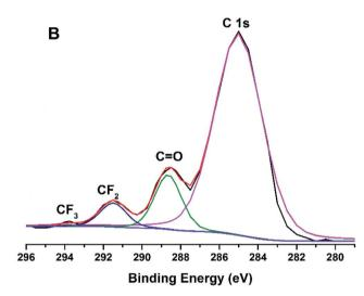
Fig. 8  $\,$  XPS C1s signals at a takeoff angle of 90  $^{\circ}$  C; (A) PU and (B) PU-F 3 (1.05 wt%).
