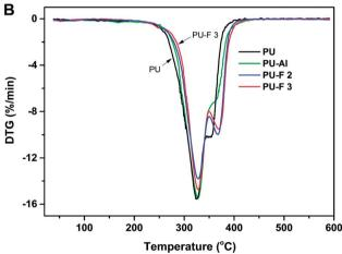
Fig. 7 TGA (A) and DTG (B) curves of PU, PU-Al (wt% = 1.86%), PU-F 2 (wt% = 0.71%) and PU-F 3 (wt% = 1.05%).
