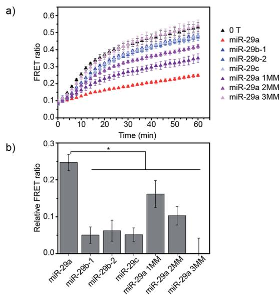
Fig. 4 Evaluation of the specificity of the miRNA detection assay. (a) FRET signal traces over time in the presence of various miRNA sequences added to DiD liposomes at a concentration of  $7.6 \times 10^{-9}$  M. (b) Corresponding bar chart representing the FRET ratio value for each miRNA sequence after 30 min of mixing DiI and DiD liposomes at 37 °C (liposome concentration of  $1 \times 10^{-4}$  M) ( $n = 3$ ,  $*p < 0.05$  (ANOVA followed by Tukey *post-hoc* test)).
