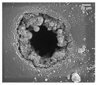
Breakdown zones of a chloropropyl-functional copolymer crosslinked into elastomers (details of elastomers in article).<sup>36</sup> Reproduced from ref. 14 with permission from the Technical University of Denmark (DTU), copyright 2017.
