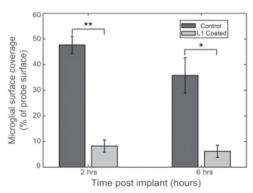
Fig. 8 Coating of biomolecules on the electrode. Effect of L1 coating to prevent microglial surface coverage following 2 hours and 6 hours implantation of neural probe. Reproduced with permission from ref. 136. Copyright 2017 Elsevier.
