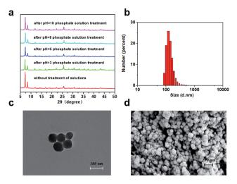
Fig. 1 (a) PXRD patterns for the as-synthesized samples of MOFs and the stability of the nano-MOFs in biological environments (red line, green line, blue line, light blue line and orange red line are the PXRD patterns for MOFs treated with PBS (2 mM) of pH 3, 5, 8 and 10 in 72 hours, respectively). (b) DLS image of the MOFs; (c) TEM image of the MOFs, scale bar  $= 100 \, \text{nm}$ ; (d) SEM image of the MOFs, scale bar  $= 200 \, \text{nm}$ .
