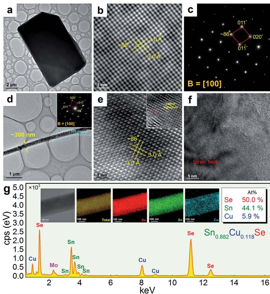
Fig. 3 (a) TEM image of a typical SnSe microplate for  $x = 0$ , corresponding (b) HRTEM image and (c) SAED pattern taken from the plate shown in (a). (d) TEM image of a section of a typical SnSe microbelt for  $x = 0.118$ , inset showing the corresponding SAED pattern, (e) corresponding HRTEM image with a dislocation shown in the inset. (f) TEM image showing significant strain contrast. (g) EDS map and spot analysis taken from a typical SnSe microbelt for  $x = 0.118$ .
