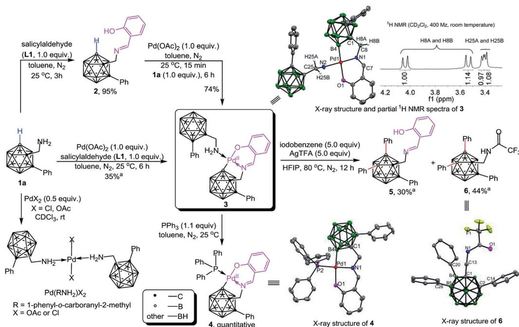
Scheme 2 Synthesis of bicyclic palladium complex **3** through palladium-mediated B–H activation and its further transformations including ligand exchange and subsequent diarylation. <sup>a</sup>Isolated yields based on *o*-carboranyl methylamine.
