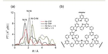
Fig. 1 (a) The  $k^3$ -weighted Fourier transform EXAFS spectra at the Ni K-edge of Ni-CTF (red), Ni-TPP (black), Ni foil (gray) and NiO (dark yellow), and (b) an illustration showing the Ni sites in Ni-CTF (weakly adsorbed molecules in electrolyte, such as water and ethanol used for the preparation of electrode, are not shown for clarity).
