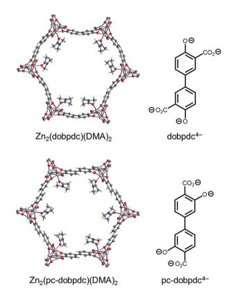
Fig. 11 Single-crystal X-ray diffraction structures of  $Zn_2(dobpdc)(DMA)_2$  (top) and  $Zn_2(pc-dobpdc)(DMA)_2$  (bottom) collected at 100 K.<sup>14b</sup> The structures of the ligands are included for comparison. Light blue, grey, red, dark blue, and white spheres correspond to Zn, C, O, N, and H, respectively. DMA = N,N-dimethylacetamide.
