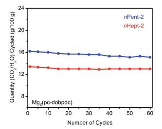
Fig. 14 Cycling stability of  $1^{\circ}$ , $2^{\circ}$ -alkylethylenediamine-appended variants of Mg<sub>2</sub>(pc-dobpdc) in a simulated CCS process. Adsorption conditions: humid 15% CO<sub>2</sub> in N<sub>2</sub>, 40 °C, 5 min; desorption conditions: humid CO<sub>2</sub>, 140 °C, 5 min. Over 60 cycles, the diamine loadings decreased by 5% for *n*Pent-2 and <1% for *n*Hept-2.
