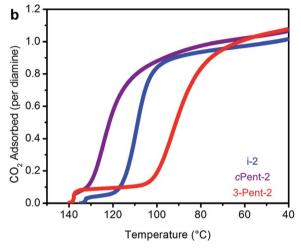
Fig. 12 Pure  $CO_2$  adsorption isobars for a series of  $1^{\circ},2^{\circ}$ -alkylethylenediamine-appended variants of  $Mg_2$ (pc-dobpdc) bearing (a) linear and (b) branched alkyl groups. In both plots, the gradient from blue to red reflects the increasing size of the substituent on the secondary amine.
