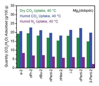
Fig. 4 Summary of the adsorption capacities from Fig. 3 at 40  $^{\circ}$ C for a series of 1 $^{\circ}$ ,2 $^{\circ}$ -alkylethylenediamine-appended variants of Mg<sub>2</sub>(dobpdc) under dry CO<sub>2</sub> (green), humid CO<sub>2</sub> (blue), and humid N<sub>2</sub> (purple).
