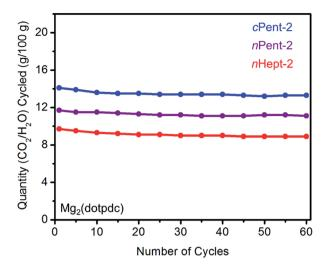
Fig. 10 Cycling stability of  $1^{\circ}$ , $2^{\circ}$ -alkylethylenediamine-appended variants of Mg<sub>2</sub>(dotpdc) in a simulated temperature swing adsorption process. Adsorption conditions: humid 15% CO<sub>2</sub> in N<sub>2</sub>, 40 °C, 5 min; desorption conditions: humid CO<sub>2</sub>, 140 °C, 5 min. Over 60 cycles, the diamine loadings decreased by 10%, 3%, and 3% for cPent-2, nPent-2, and nHept-2, respectively.
