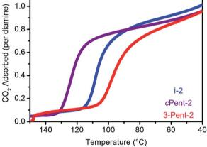
Fig. 8 Pure  $CO_2$  adsorption isobars for a series of  $1^{\circ},2^{\circ}$ -alkylethylenediamine-appended variants of  $Mg_2$ (dotpdc) bearing (a) linear and (b) branched alkyl groups. In both plots, the gradient from blue to red reflects the increasing size of the substituent on the secondary amine.
