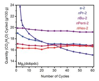
Fig. 5 Cycling stability of  $1^{\circ}$ , $2^{\circ}$ -alkylethylenediamine-appended variants of Mg<sub>2</sub>(dobpdc) in a simulated temperature swing adsorption process. Adsorption conditions: humid 15% CO<sub>2</sub> in N<sub>2</sub>, 40 °C, 5 min; desorption conditions: humid CO<sub>2</sub>, 140 °C, 5 min. Over 60 cycles, the diamine loadings decreased by 13%, 23%, 11%, 3%, and 1% for e-2, nPr-2, nBu-2, nPent-2, and nHex-2, respectively.
