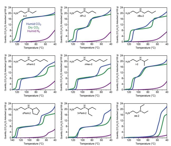
Fig. 3 Dry  $CO_2$  (green), humid  $CO_2$  (blue), and humid  $N_2$  (purple) adsorption isobars for a series of  $1^{\circ}$ ,  $2^{\circ}$  -alkylethylenediamine-appended variants of Mg<sub>2</sub>(dobpdc), as well as ee-2-Mg<sub>2</sub>(dobpdc) for comparison.
