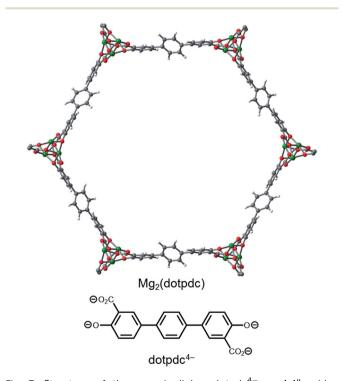
Fig. 7 Structure of the organic linker dotpdc<sup>4-</sup> = 4.4"-oxido-[1,1':4',1"-terphenyl]-3,3"-dicarboxylate and a model of the hexagonal pore of Mg<sub>2</sub>(dotpdc). Green, grey, red, and white spheres correspond to Mg, C, O, and H, respectively.
