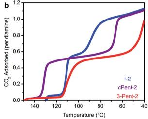
Fig. 2 Pure CO<sub>2</sub> adsorption isobars for a series of 1°,2°-alkylethylenediamine-appended variants of Mg<sub>2</sub>(dobpdc) bearing (a) linear and (b) branched alkyl groups. The lower temperature CO2 adsorption step moves to successively lower temperatures as the substituent size increases. In both plots, the gradient from blue to red reflects the increasing size of the substituent on the secondary amine.
