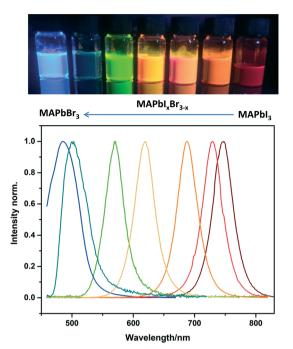
Fig. 4 Photo of sample vials under UV illumination and PL spectra of MAPbl<sub>x</sub>Br<sub>3-x</sub> perovskite NCs in toluene with different halide compositions.
