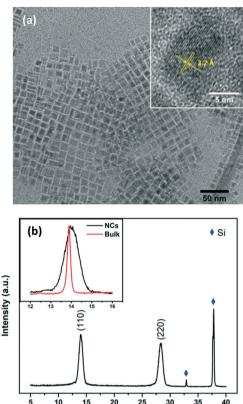
Fig. 2 (a) TEM images of MAPbl<sub>3</sub> NCs stored for over 8 months. The inset is the high resolution TEM of a typical NC. The interplanar spacing was measured to be 3.2 Å, which is consistent with the (220) plane of tetragonal phase MAPbI<sub>3</sub> perovskite.<sup>26</sup> (b) XRD patterns of MAPbl<sub>3</sub> NCs coated on silicon wafer. The inset is the comparison of the (110) peak of MAPbl<sub>3</sub> NCs with that of the bulk film.
