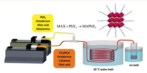
Fig. 1 Schematic diagram of the flow reactor system used for the synthesis of MAPbX<sub>3</sub> nanocrystals at low temperature
