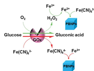
Scheme 1 Illustration for the proposed colorimetric biosensor method for detection of glucose.
