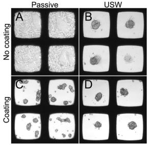
Fig. 5 Bright field microscopy images of HepG2 cells cultured in the multi-well microplate with and without coating or ultrasound. Four conditions: 48 hours of passive culture in an un-coated microplate (A), 24 hours active + 24 hours passive culture in uncoated microplate (B), 48 hours of passive culture in a coated microplate (C) and 24 hours active + 24 hours passive culture in a coated microplate (D). Each micro-well is 350 µm wide.
