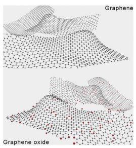
Fig. 11 Schematic illustration of single-atom layer graphene and graphene oxide.
