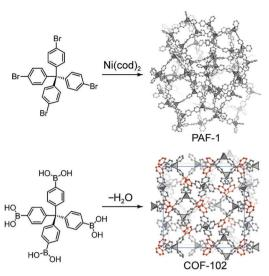
Fig. 10 Schematic representation of the synthesis of PAF-1 (top) and COF-102 (bottom).<sup>204,208</sup> Gray, red, and orange spheres represent C, O, and B atoms, respectively; quaternary carbon atoms are shown as grey tetrahedra and H atoms of the triphosphine ligands are omitted for clarity.
