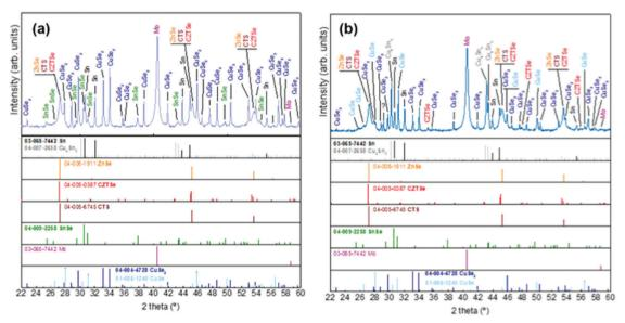
XRD diffractograms of samples without Ge at t1 (a) and with Ge (25 nm below the CTZ precursor) at t1 (b)
