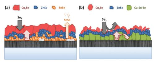
Scheme 2 Schematic sketches of the different intermediate steps and reaction mechanisms involved in the formation of CZTSe during the selenization of metallic Cu-Zn-Sn precursors: (a) reference sample without Ge, and (b) Ge-containing sample.
