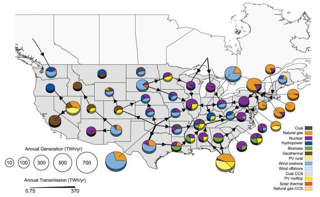
Fig. 3 Geographical breakdown of the U.S. cost-optimal electricity system in 2030 for solution B (full cooperation in Fig. 1). The size of the pie charts is proportional to the electricity generation in each state (TWh per year) whereas the slice colours denote the technology and the slice sizes represent the associated percentage share. Arrows illustrate the electricity trade between the U.S. states and Canada, with their thickness proportional to the amount of electricity traded.
