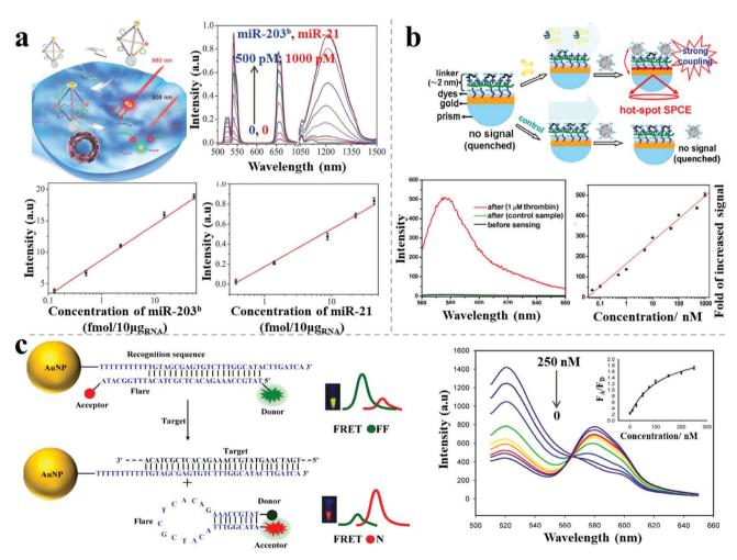
Fig. 9 Photoluminescence-based sensors. (a) Plasmonic hybrid NP pyramids and luminescent recovery effect for intracellular dual microRNA quantitation. (b) AgNP-dyes-Au film assemblies and hot-spot induced emission for thrombin detection. (c) AuNP-based FRET nanoflares and fluorescence response for intracellular mRNA detection. Reproduced with permission: ref. 14 Copyright 2017 Wiley-VCH Verlag GmbH & Co.; ref. 48 and 49 Copyright 2014, 2015 ACS.
