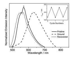
Fig. 7 Normalized emission spectra of 6 in powder, ground and fumed forms (the asterisk indicates an instrumental artifact). The inset shows the emission wavelength of the repeated mechanochromic behavior of 6.
