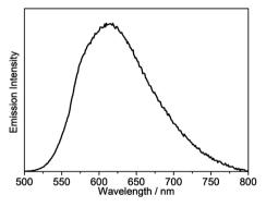
Emission spectrum of 8 in dichloromethane at 298 K.
