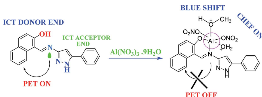
Fig. 8 Probable mechanistic pathway for sensing Al(III) ions. 108
