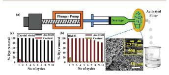
Fig. 20 (a) Schematic of flow device developed for adsorption (inset shows SEM image of filter); (b) and (c) recyclability studies of Rh123 and crystal violet, respectively.<sup>84</sup>
