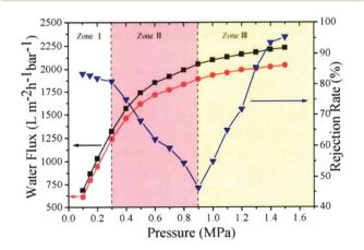
Fig. 24 Pressure-dependent flux and rejection of EB molecules of NSC-GO membrane under different pressure.<sup>85</sup>
