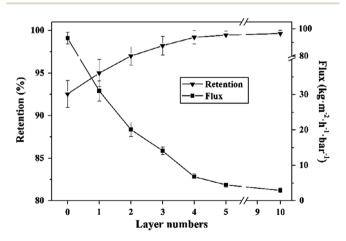
Fig. 9 Effect of layer numbers on separation performance of PDDA/ GO membrane.69
