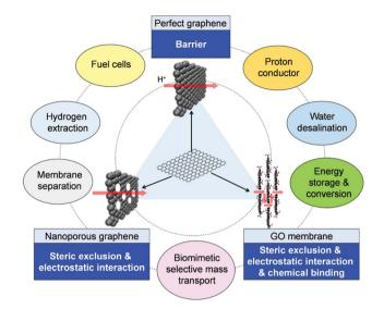
Fig. 4 Schematic illustrating the structure of graphene, NG and GO membrane, the mechanism for selective mass transmembrane transport and possible uses.52
