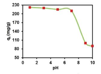
Fig. 16 Effect of solution pH on adsorption capacity.<sup>79</sup>
