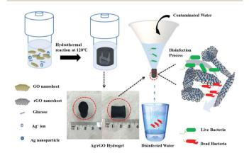
Fig. 13 Synthesis and application of Ag/rGO hydrogel as bactericidal filter for point-of-use water disinfection.<sup>76</sup>
