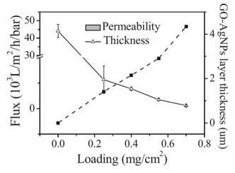
Fig. 12 Variations of GO-AgNP layer thickness and pure water permeability as a function of GO-AgNP loading on membrane.<sup>64</sup>
