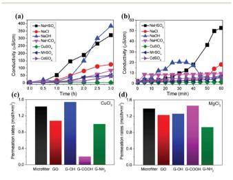
**Fig. 6** (a) Penetration processes of different ionic compounds through graphene oxide membranes;<sup>57</sup> (b) initial stages of the penetration processes;<sup>57</sup> (c) Cu<sup>2+</sup> and (d) Mg<sup>2+</sup> permeation rates through different membranes.<sup>58,59</sup>
