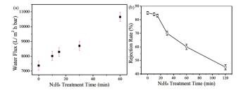
Fig. 23 (a) Water flux and (b) rejection rate of EB molecules of GO/CHNs membrane with  $N_2H_4$  treatment for different durations.<sup>85</sup>
