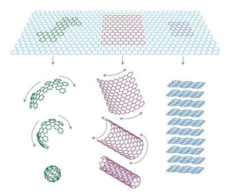
Fig. 2 Graphene is a basic building block for graphitic materials of all other dimensionalities.<sup>23</sup>
