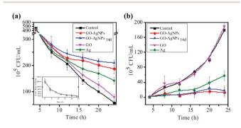
Fig. 11 (a) Flux change using *E. coli*-containing feed water under constant pressure; (b) viable cell concentration in reject water under constant flow rate.<sup>64</sup>
