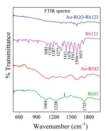
Fig. 21 FTIR spectra of Rh123 before and after adsorption on rGO–  $\mathrm{Au.^{84}}$
