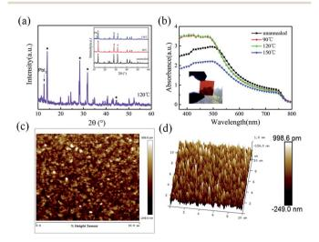
Fig. 3 (a) XRD patterns and (b) the absorption spectra of the CH<sub>3</sub>-NH<sub>3</sub>PbI<sub>3</sub> thin films after annealing at different temperature, respectively. (c) 2D, (d) 3D AFM characterizations of the LFCVD CH<sub>3</sub>NH<sub>3</sub>PbI<sub>3</sub> thin film after annealing at 120 °C on the FTO/c-TiO<sub>2</sub> substrate.
