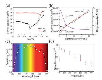
Fig. 4 (a) J-V curves of the perovskite photovoltaic device in the dark and under 650 nm irradiation. (b) Linear dynamic range of the perovskite device and the responsivity. (c) Spectral response of the perovskite photodetector. (d) The noise current of the perovskite device measured under dark condition by using a lock-in amplifier (SR830) from 150-700 Hz frequencies at zero bias.
