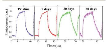
Fig. 6 Photo response behaviour of the perovskite device stored in air for 60 days.
