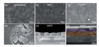
Fig. 2 SEM images of the perovskite films deposited via LFCVD procedure on FTO/c-TiO<sub>2</sub>, (a) before and after annealing at (b) 90 °C, (c) 120 °C and (d) 150 °C for 30 min, respectively. The cross-section SEM image of (e) the perovskite film after annealing at 120 °C for 30 min, (f) the multilayer structure in a complete photovoltaic structure.
