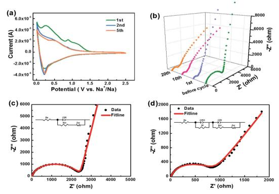
Fig. 6 (a) Cyclic voltammogram curves of sample HC-1000 at a scan rate of  $0.1 \, \text{mV s}^{-1}$  between  $0.01 \, \text{and} \, 2.5 \, \text{V}$ . (b) Nyquist plot deduced from EIS measurements of as prepared cells before cycle, after 1st, 10th and 20th cycle. (c) The fitline of Nyquist plot and equivalent circuit used to fit the EIS of sample HC-1000 before cycle and (d) after 20th cycle.
