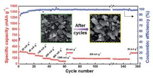
Fig. 8 Discharge capacities of HC-1000 at different current densities of 20, 40, 100, 200, 500 and 1000 mA  $\rm g^{-1}$ , respectively. A long-term cycling performance is recorded from the 70<sup>th</sup> to the 350<sup>th</sup> cycles at 200 mA  $g^{-1}$  and SEM images of the HC-1000 electrodes before and after 360 cycles.
